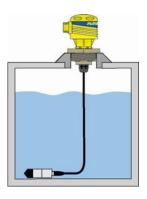
**Note:** Use caution when sealing the cable at the top of the tank. The ventilation tube must be open and free to allow air to flow back to the pressure diaphragm. Avoid blocking the ventilation tube by compressing the cable. Always keep the cable termination clean, dry and free of moisture and prevent liquid from entering the vent tube.
