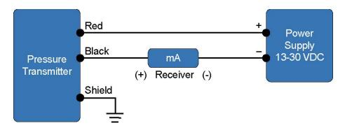
The maximum receiver load resistance (RLmax) for the DC power supply voltage (Vsup) is expressed by the formula:
