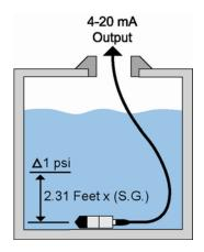
For liquids with a different SG, simply divide 2.31 by the new SG to determine the new ratio. For example, the LD32-S001 is installed in a liquid with a SG = 0.85. The new ratio is as follows:
